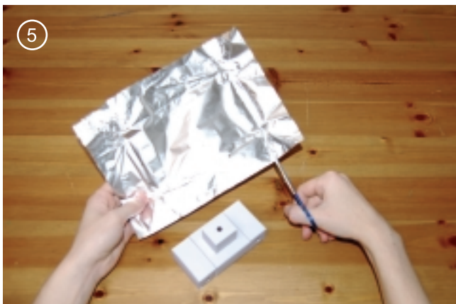
5. Parts 1, 2, 4 and 5 on the outside glue with foil. You should look at a bright light through the detail to make sure that it does not shine through.
