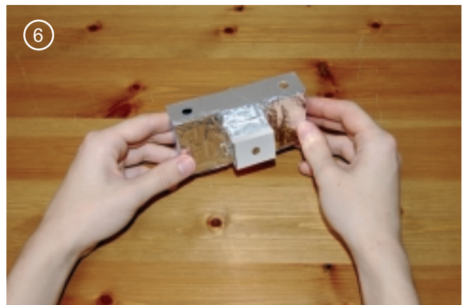
6. On top of foil you should glue part number 3, which will become part of the shutter mechanism. You should glue it not very close, so the shutter can opens and closes freely. Look at the diagram on page number 5.
